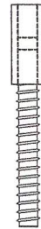
THREADED ROD WITH COUPLER 3/8"-16 and 1/2"-13 Refer to Anchor Spacing Tables for AS Part Number. See this page for coupler detail.
